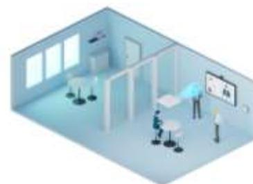
Here, TeamConnect Ceiling 2 is being used as an extender microphone for a collaboration screen. The dynamic beamforming allows for flexible usage of the complete space and collaboration with remote participants.
