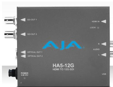
AJA's HA5-12G allows users to convert an HDMI 2.0 input to two 12G-SDI single link outputs. It includes two SDI DA outputs and transmits 12G-SDI on each SDI link, reducing cable runs when transporting 4K/UltraHD SDI. HA5-12G supports up to 8-Channels of audio from the HDMI source or 2-Channel analog audio (RCA), with eight or two channels of digital embedded audio on 12G-SDI.
