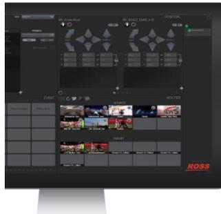
interface. The application provides seamless integration with tracking systems and real-time 3D rendering engines such as XPression and Frontier. It comes installed on a touchscreen PC for virtual set camera calibration, scene manipulation, media replacement, event triggering, animation control, robotic camera movement control and more.
