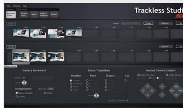
in order to create movement. They use a stationary physical camera, with all the camera movement being done within the graphics engine. This eliminates the need for physical tracking equipment.
